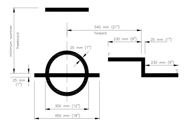
Figure 2 – Lines to be used with the Load Line Mark
