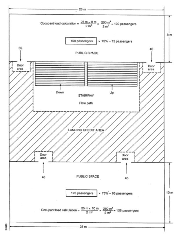
Figure 3 – Occupant loading calculation example
